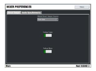
**Global Direct Output Source** Open the drop down menu and select the point in the channel signal path to feed the direct outputs. The list is in signal processing order. The setting affects all 64 input channel direct outputs.
